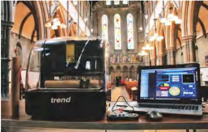
▲ Pic.19 The handles were placed into the Trend CNC machine for engraving
